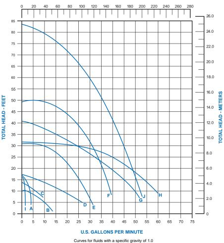
The above performance curves are designed to serve as a reference guide for locating a pump with the approximate performance range to meet your application (please consult the factory with exact application specifications). Each individual pump series is identified in the chart for each corresponding curve.
